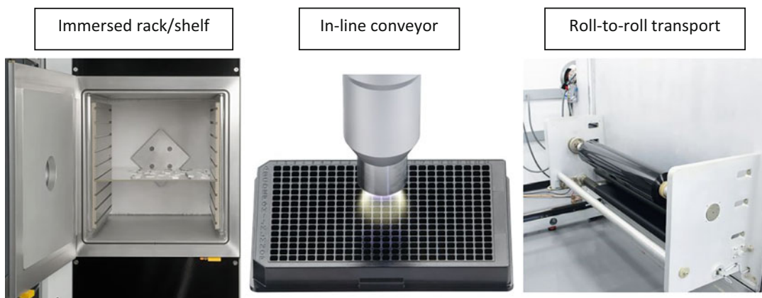
Fig. 2 System configurations shown from left to right: Plasmatreat Aurora 350, Plasmatreat RD1004, and Plasma Science roll-to-roll system
