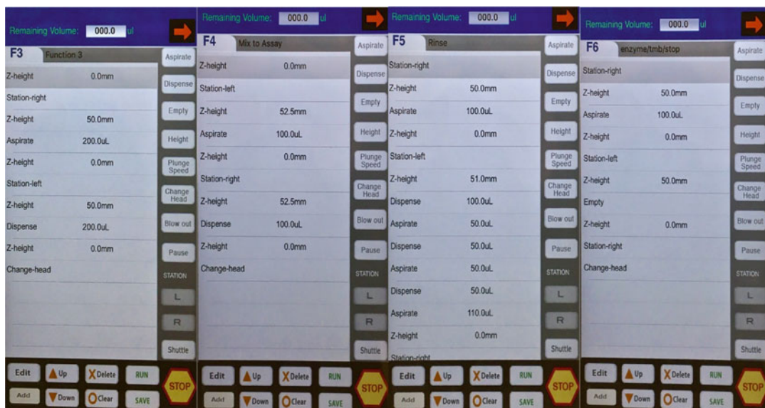
Fig. 10 iPipette functions 3–6 for running ELISA. Comprising transferring of the diluent to the HELICA mixing plate, introducing the samples and standards, transferring the solution to the ELISA plate, rinsing, and adding enzyme, substrate and stop solution.
