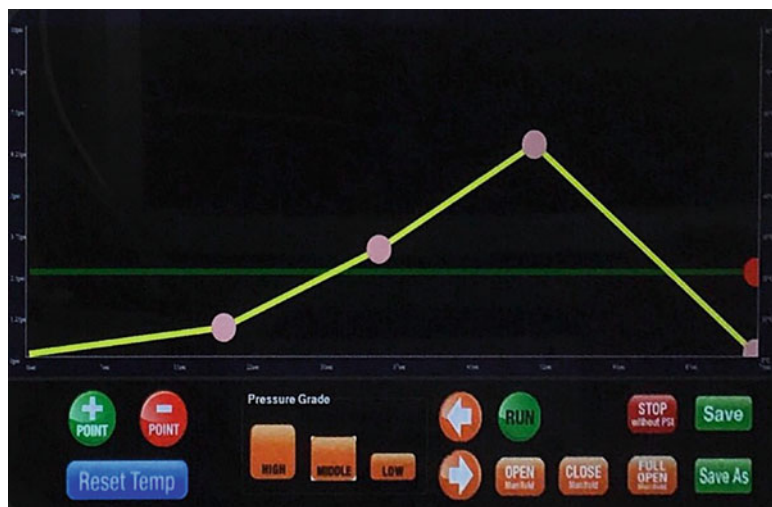
Fig. 3 Pressure profile for the conditioning of the column with methanol
