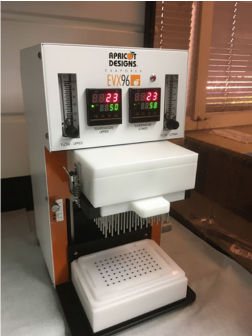
Fig. 7 The EVX96 used for the second experiment using methanol solutions to optimize evaporation techniques
