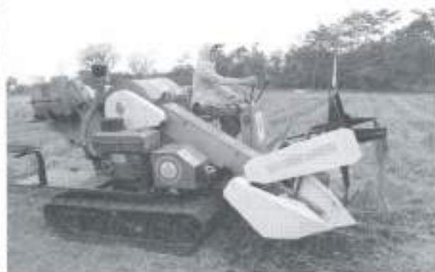
Gambar 8.9. Mesin panen padi riding type (*Indo-Combine Harvester*)
