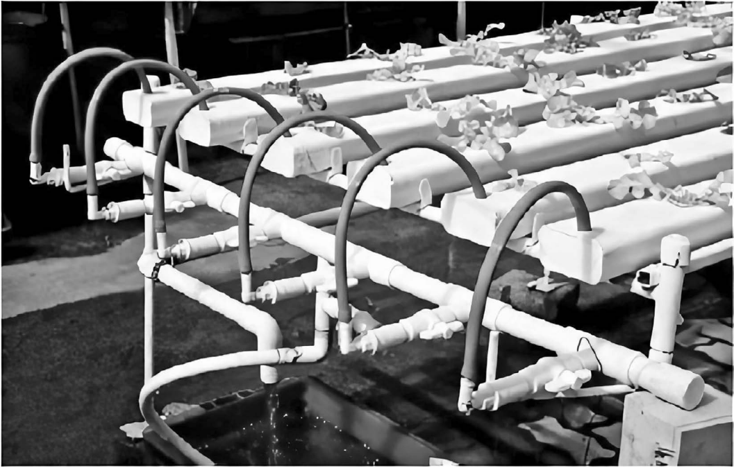
FIGURE 2.5 Depiction of the continual flow solution method.
