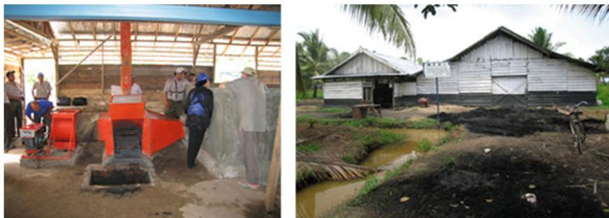
**Fig. 2.3** First pilot project flatbed dryer using husk energy at Upang Village, Banyuasin
