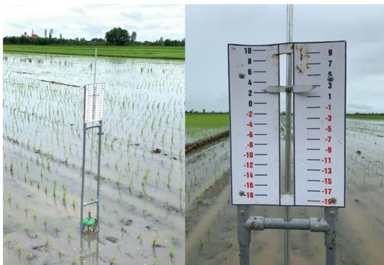
**Fig. 5.1** Modified Alternate-wetting-and-drying (AWD) tube using buoyancy to show the water level
