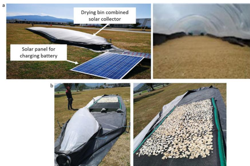
**Fig. 4.12** Types of dryers **a** Solar bubble dryer for paddy drying, **b** Solar bubble dryer for mushroom drying
