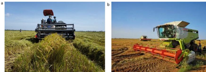
**Fig. 4.11** Small and big scale combine harvester **a** Small and medium scale combine harvester, lower than 2 ha per hour, **b** Big scale combine harvester, higher than 2 ha per hour
