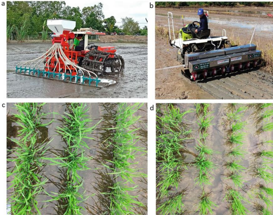
**Fig. 4.9** Typical wet-mDSR machines being tested in the MRD **a** Line seeder, **b** Hill seeder, **c** Seedlings at 20 days after line seeding **d** seedlings at 20 days after hill seeding
