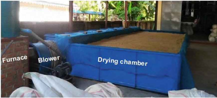
a Flatbed dryer used for paddy grain drying
