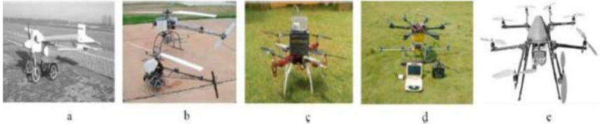
Gambar 3. Jenis Drone a. Fixed Wing, b. Rotor tunggal, c. Quad copter, d. Hexa copter, e. Octo copter (Mogili dan Deepak 2018)
