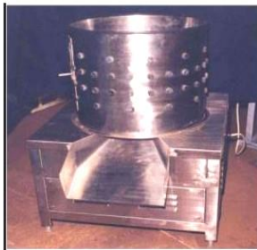
Plucker (TP) : Dimensi total P x L x T = 80 x 80 x 100 cm, Drum berdiameter 60 cm Kapasitas 10 ekor/proses, Motor 2 HP Rp 15.500.000,-/unit
