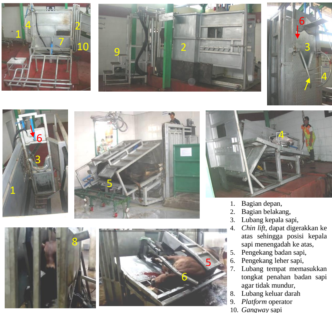
Gambar 96. Restraining Box Tipe Putar Hidrolik / Mark-4 (b).
