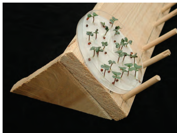
FIGURE 9.12 Wooden apparatus for holding Petri dishes at a 45° angle. (Courtesy of Brian R. Cody.)
