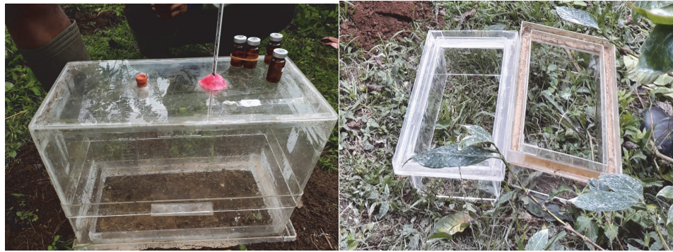
Gambar 2. Sungkup tertutup (kiri) dan penampang sungkup (kanan) Figure 2. Close chamber (left) and the chamber base (right)
