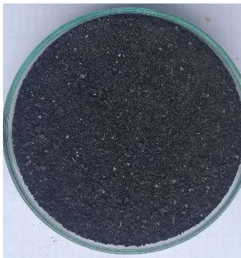
Abu boiler kelapa sawit
