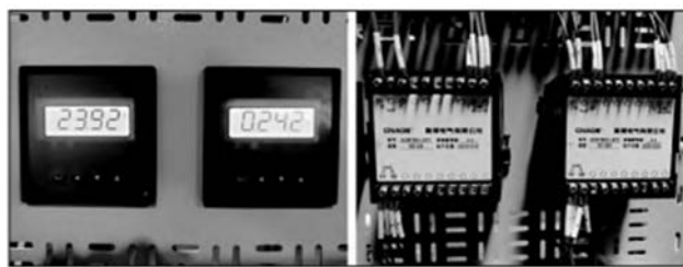
Figure 1. Smart instrument (digital voltmeter, digital ammeter), physical, wiring diagram.
