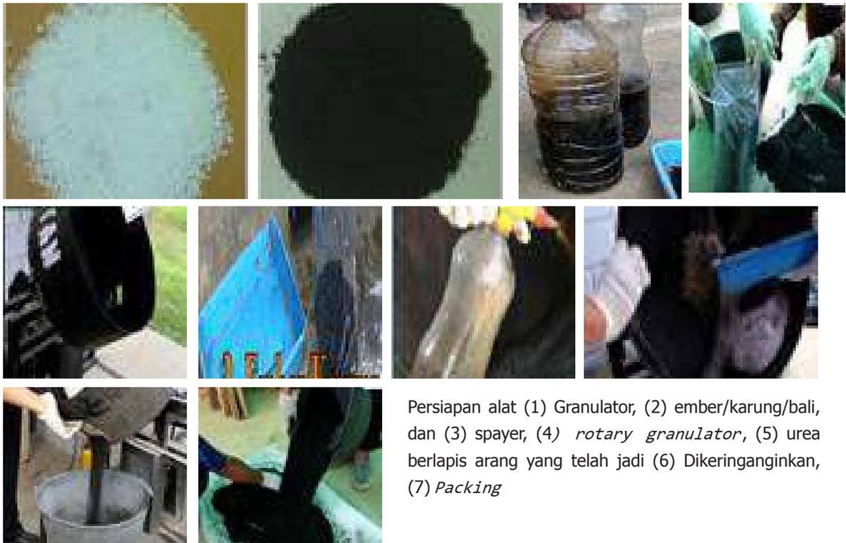
Persiapan alat (1) Granulator, (2) ember/karung/bali, dan (3) spayer, (4) *rotary granulator*, (5) urea berlapis arang yang telah jadi (6) Dikeringanginkan, (7) *Packing*
