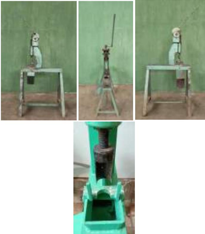
**Gambar 5.2** Alat Pemotong *Bud Chip* Tipe Meja
