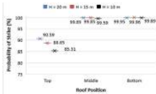
Figure 6. Probability of a lightning strike to the rim edge of the tank cylinder.
