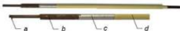
Figure 1. The structure of the Arcair Sea-Weld electrode; a – electrode core wire, b – iron oxide layer, c – aluminum covering, d – plasticized vinyl.
