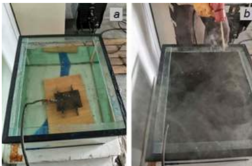
Figure 2. The experimental aquarium used for simulating underwater welding; a – before burning of an electrode, b – after burning of an electrode (60 sec).
