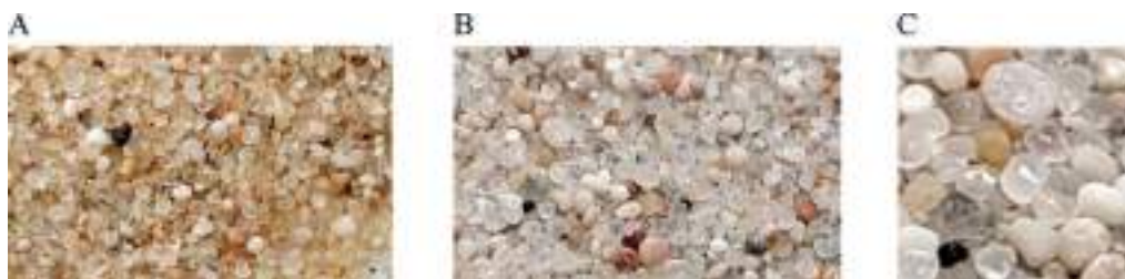
Figure 1. Grains of desert sand before (A) and after bioleaching (B), details of corrosive holes after bioleaching (C).
