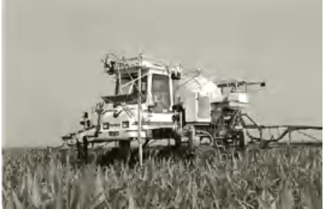
FIGURE 4.13 An example of an intelligent variable-rate applicator. The machine-mount crop sensing system is capable of self-calibrating to natural lighting conditions.
