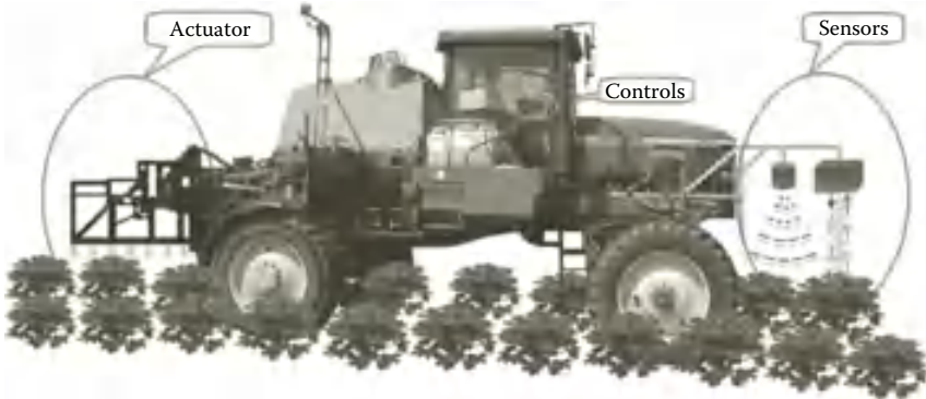
FIGURE 6.2 Illustration of a sensor-based variable-rate application system including sensors, controls, and the actuator.
