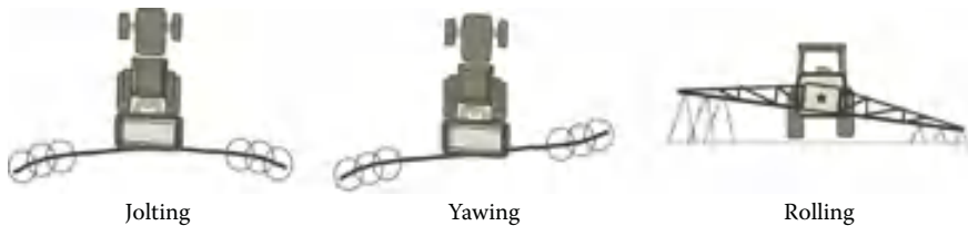
FIGURE 4.14 A few scenarios of unwanted sprayer boom vibrations or waving. (Data courtesy of Professor J. De Baerdemaeker.)
