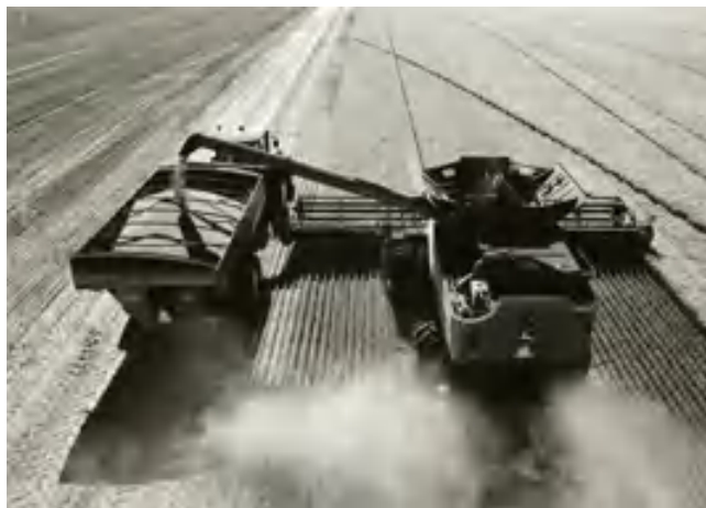
FIGURE 5.9 John Deere’s Machine Sync that can synchronize the operation of combines and tractors with grain carts for “on-the-go” harvesting. (Photo courtesy of Deere & Company.)
