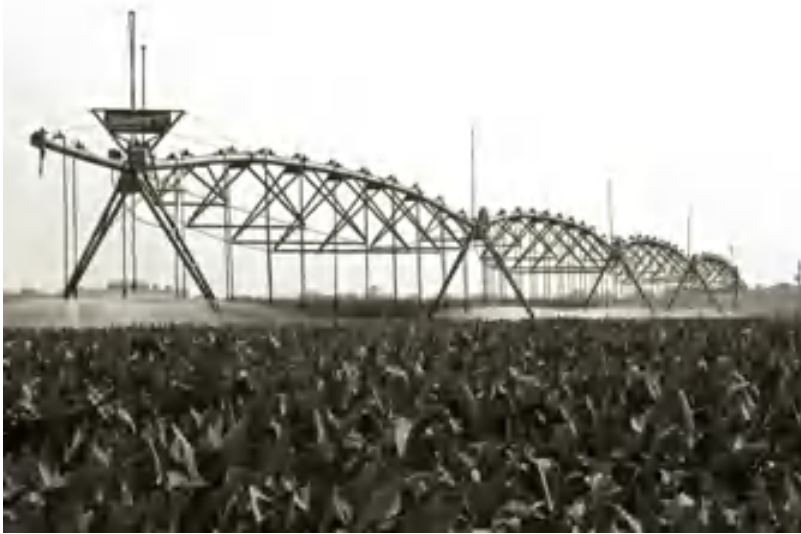
FIGURE 6.4 A center pivot variable-rate irrigation system running at the research farm of USDA-ARS Crop Production Systems Research Unit in Stoneville, Mississippi, USA.
