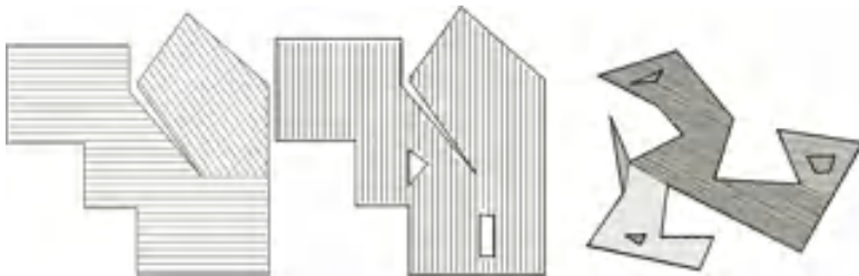
FIGURE 5.6 Examples of an optimized coverage path planning algorithm based on a headland turning cost function and a divide-and-conquer strategy for 2D terrains, where the inner polygons indicate nontraversable obstacles. (From Jin, J. and L. Tang. 2006. Optimal Path Planning for Arable Farming , ASABE Paper Number 061158, ASABE, St. Joseph, MI, USA; Jin, J. and L. Tang. 2010. Transactions of the ASABE , 53:283–295. With permission.)
