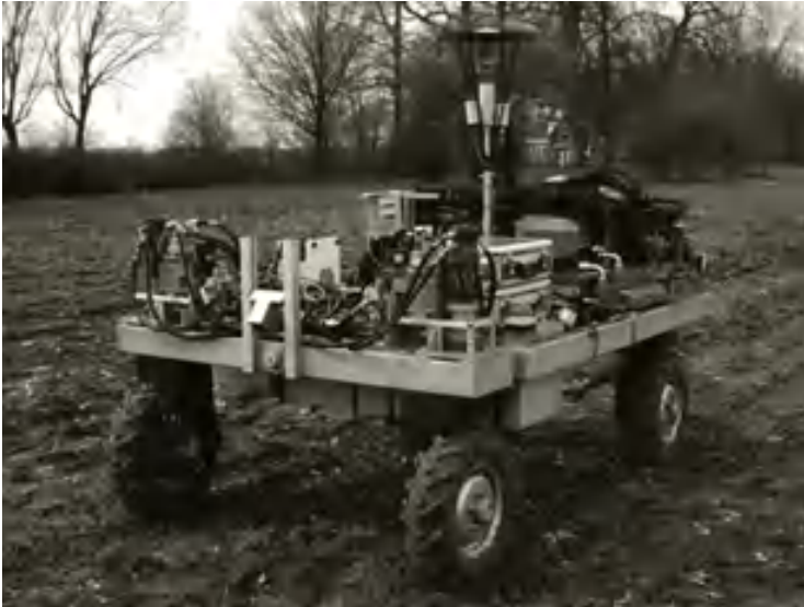
FIGURE 5.16 A weeding robot developed at Wageningen University. (From Bakker, T., J. Bontsema, and J. Müller. 2010a. Journal of Terramechanics , 47:63–73. With permission.)
