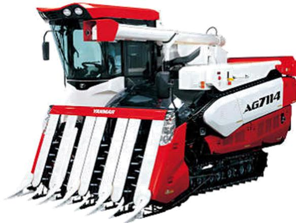
Gambar 3. Head feed type combine harvester
